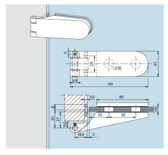
Hinge with frame pivot for wooden frames,
