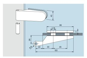
Hinge with frame pivot, complete with sleeve, rebate depth 26 mm, extended colour options, door weight max. 45 kg
