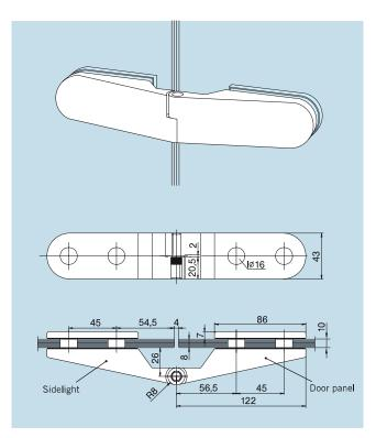
Hinge for mounting onto sidelight, stainless steel pin, door weight max. 35 kg Art. No. 10.245  $\mbox{L}$  (as illustr.) Art. No. 10.247  $\mbox{R}$  Weight in kg: alumin. 0.557
