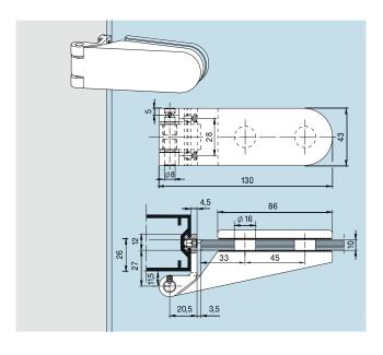
Hinge with frame pivot for aluminium frames, stainless steel pin, door weight max. 35 kg
